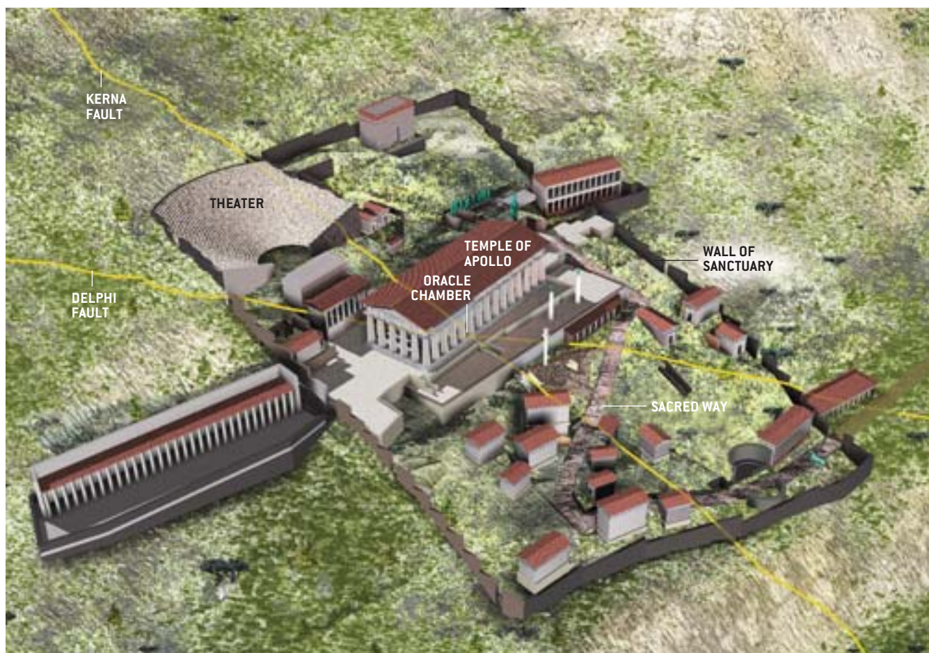
TWO GEOLOGIC FAULTS intersect under the Temple of Apollo at Delphi (above and details on opposite page). This intersection made the rock more permeable and provided pathways (visible in cutaway) along which both groundwater and gases were able to rise. Tectonic activity heated the
